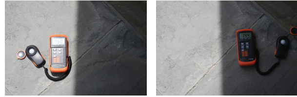
(a) Direct Sunlight: 96,000 lux (b) Within Shadow 14,400 lux
