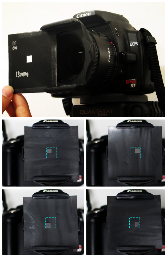
Figure 1. (Top) Modified filter-holder on a Canon Digital Rebel XT SLR camera accepts different masks slid in front of the lens. (Bottom) Four masks mounted on the camera to obtain 2 \times 2 resolution enhancement.
