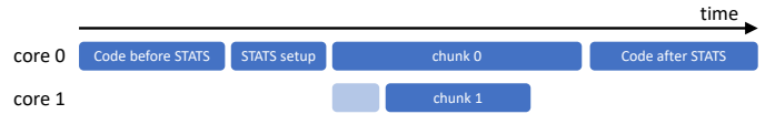
Fig. 8: Sequential code outside the code region of STATS does not benefit from the additional TLP that STATS generates.
