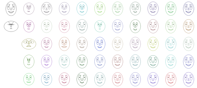
Figure 6: Chernoff Face View for monitoring. Note that the two faces in the first column are reference faces for showing two extremes, The first happy face is the reference for the all zero data input, and the second angry and unhappy face is for an imaginary input data with highest values input for each time bin within the current time window. The color of each face is consistent with previous views. As we discovered in Figure 5 the high value data outlier is the third object. In this visualization, we can also pick out this outlier easily, the third face in the second column is indeed an outlier visually.
