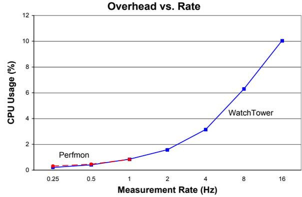
Figure 3: Overhead vs. rate with 256 counters for Perfmon and WatchTower. Note that the Perfmon line does not extend beyond 1 Hz.
