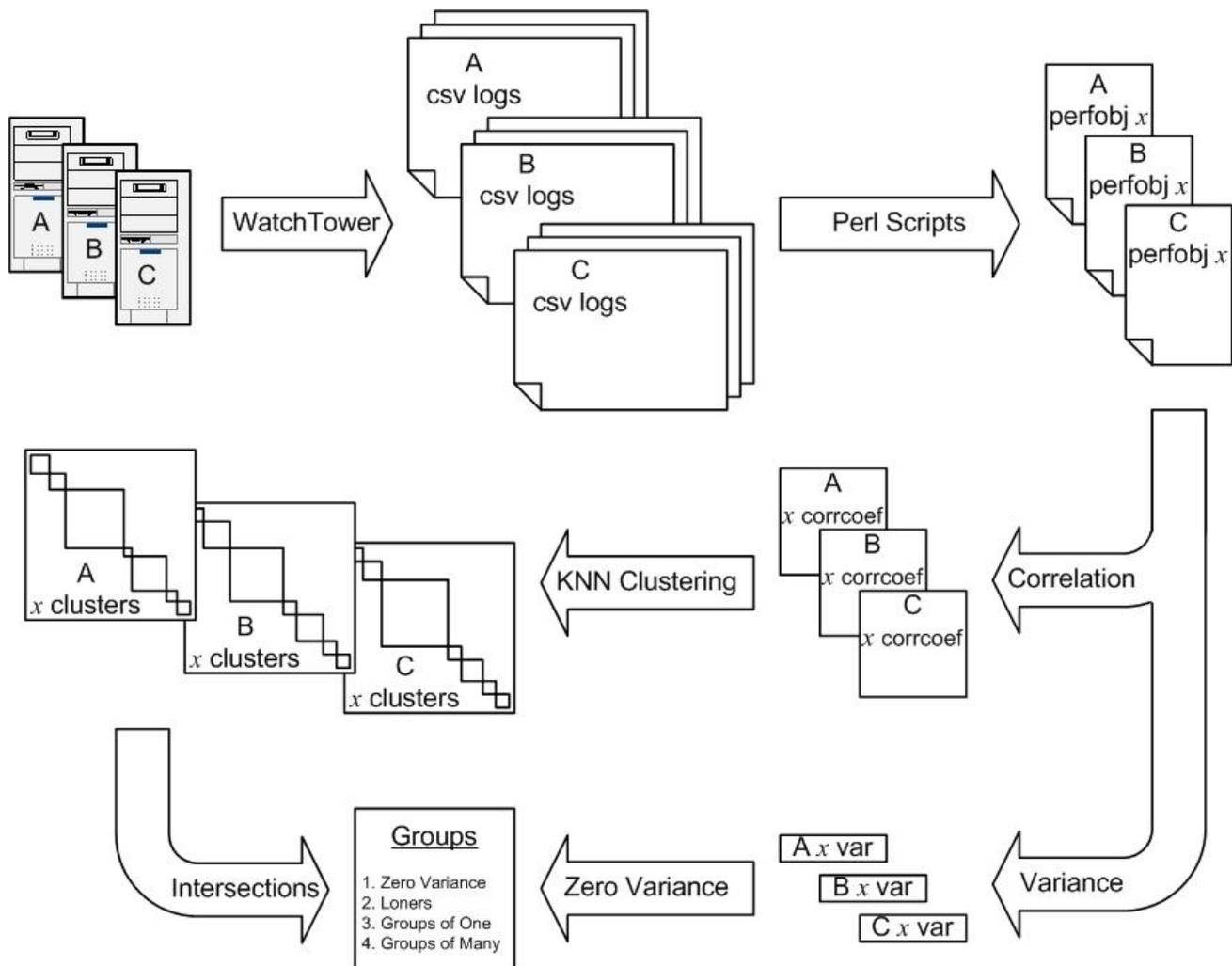
Figure 4: Graphical representation of the current correlation elimination data reduction process.
