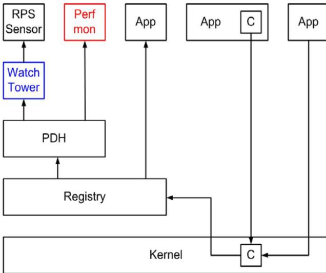
Figure 1: Windows performance monitoring structure.
