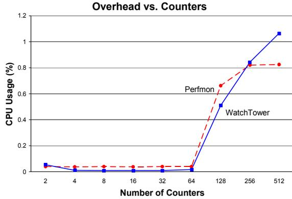
Figure 2: Overhead vs. counters at 1 Hz for Perfmon and WatchTower.
