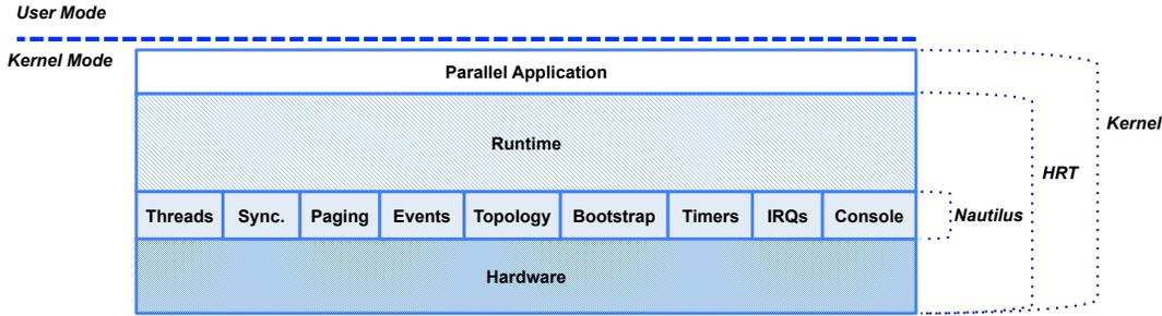
Figure 2: Structure of Nautilus.
