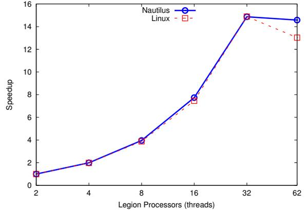
Figure 12: Speedup of Legion (normalized to 2 Legion processors) circuit simulator running on Linux and Nautilus as a function of Legion processor (thread) count.
