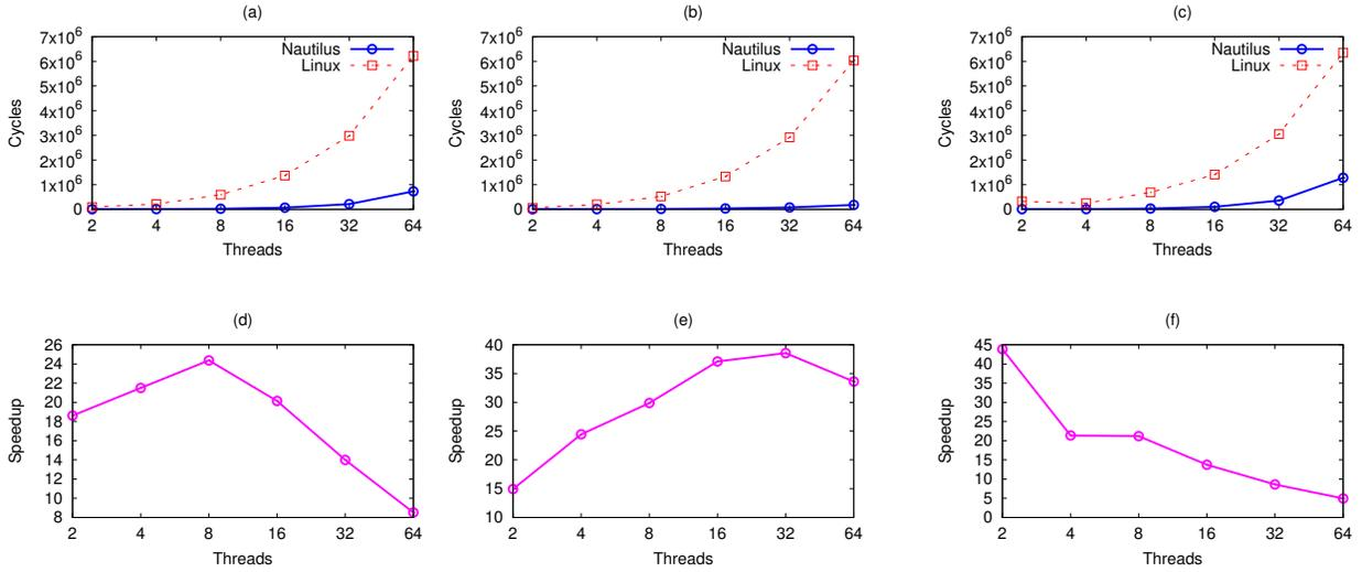
Figure 4: Average (a), minimum (b), and maximum (c) time to create a number of threads in sequence. Average (d), minimum (e), and maximum (f) speedup of Nautilus over Linux for multiple thread creations.
