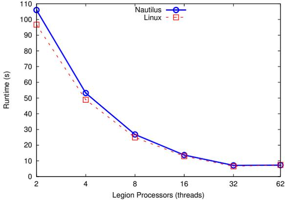
Figure 11: Run time of Legion circuit simulator versus core count. The baseline Nautilus version has higher performance at 62 cores than the Linux version.
