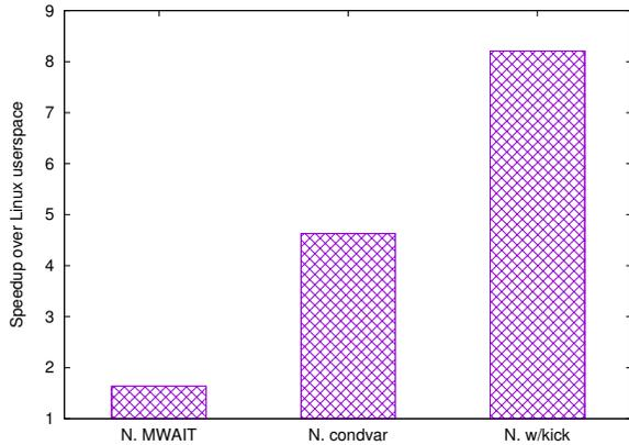
Figure 7: Speedup over Linux for event wakeups in Nautilus.
