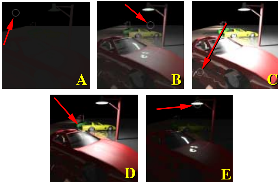
Fig. 10. Example display images from the interactive foveal display program: each red arrow points to the foveal neighborhood, a circled region around the user's direction of gaze. A) Placing the circled region on the night sky causes adaptation luminance L_{wa} near the absolute threshold of vision where contrast sensitivity is extremely low causing the anomalously dim street light. B) Adapting to distant terrain lit by moonlight greatly increases contrast sensitivity, causing contrast compression in the foreground. C) Directing attention to the deep car shadows in the foreground reveals reflected details of the wet ground below the car. D) Adapting to the distant yellow car shows its reflection on wet pavement. E) Gazing at the bulb of the streetlight causes extremely high adaptation luminance, darkening the rest of the scene. Images A) and E) illustrate the limitations of globally applied adaptation models; local adaptation in the human visual system ensures that the street light and car have a bright appearance for any direction of gaze in the scene.
