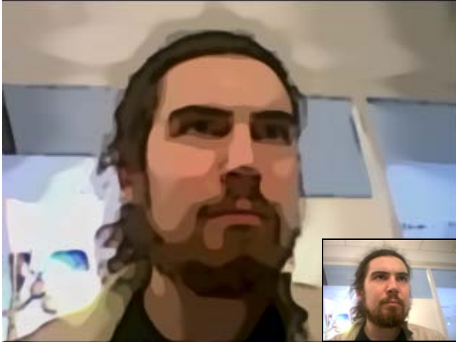
Figure 1: The GPU implementation of our system can be connected to a video capture source (such as a webcam), creating a real-time stylization effect. Demos and project information are available at: http://videoabstraction.net/
