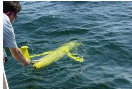
Webb Research glider (electric): 0.2-0.4 m/s, \sim 1 month; Hotel + Propulsion: \sim 2\text{W}
