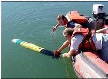
REMUS: 1.0-2.9 m/s, 5-20 hours Hotel load: \sim 30\text{W} Propulsion: 15-110\text{W}
