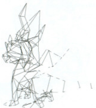
3.6.4 The real-time model of Spyro the Dragon ™ has 352 polygons and 230 vertices. The modeling started in Alias Power Animator 8.5 with a couple of polygonal geometric primitives and continued by pulling points. Individual polygons were added for features like the eyes, feet, and interstices between joints. ( Spyro the Dragon ™ . Images Courtesy of Universal Interactive Studios, Inc. and Insomniac Games, Inc.)
