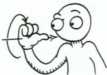
3.4.5 In a right-handed coordinate system the direction in which your hand closes to make a fist is the direction of a positive rotation around any axis represented by the extended right-hand thumb.
