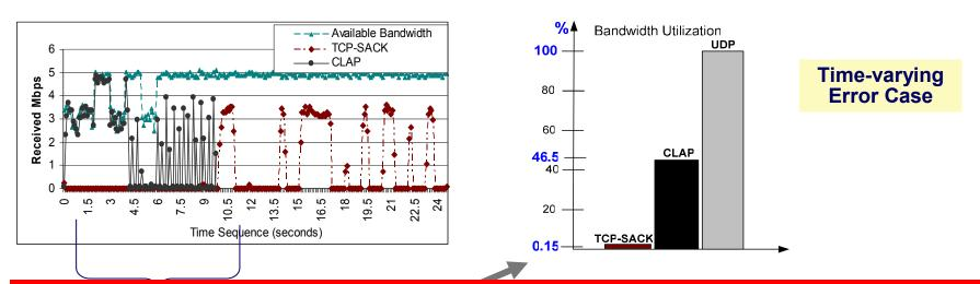
TCP shuts down operation in the presence of time-varying link errors.
