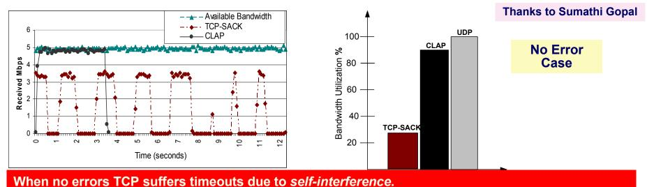
CLAP gains 300% over TCP-SACK, making far better utilization of link bandwidth
