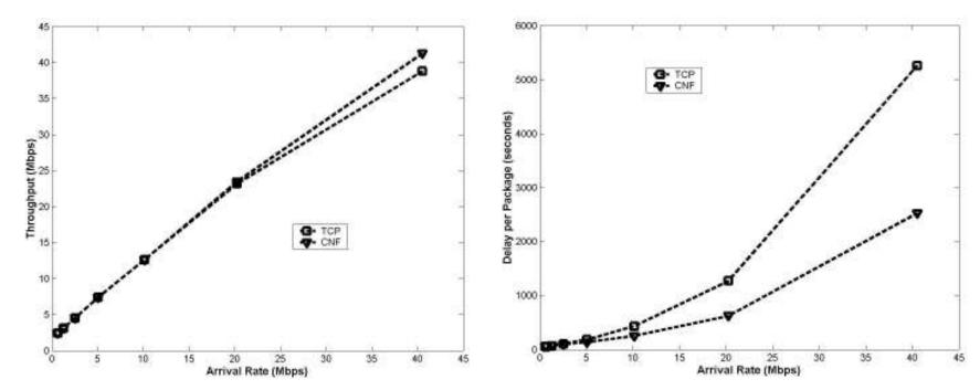
CNF starts to outperform TCP in terms of throughput for On-OFF traffic as the overall arrival rate increases End-to-end delay for CNF is lower than that for TCP for On-OFF traffic and the difference increases as the overall arrival rate increases
