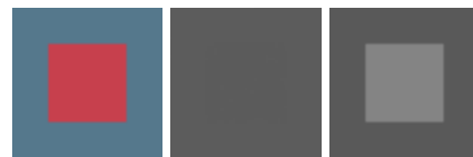
Figure 2: Isoluminant changes are not preserved with traditional color to grayscale conversion. Converting an image of a reddish square whose luminance matches that of the blue background (Left) to grayscale (Middle) results in a featureless gray image. The Color2Gray algorithm incorporates chrominance changes (Right).
