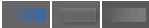
Figure 7: Left : Equiluminant fade from gray to blue on a background with the same luminance. Middle : Color2Gray result with \mu = 9 neighborhood. Right : Color2Gray result with a full neighborhood ( \theta = 270^\circ ; \alpha = 8 ). Using a small neighborhood produces a dark band through the middle of the fade and produces artifacts where the edge of the fade meets the background; whereas using the entire set of pixels as the neighborhood (full neighborhood) preserves the horizontal fade with respect to its background.
