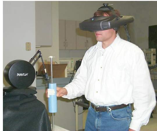
Figure 1: Mechanism for allowing a subject to manipulate the virtual world. The task was to lower a virtual cylinder as close to a virtual table as possible without contacting the virtual table.
