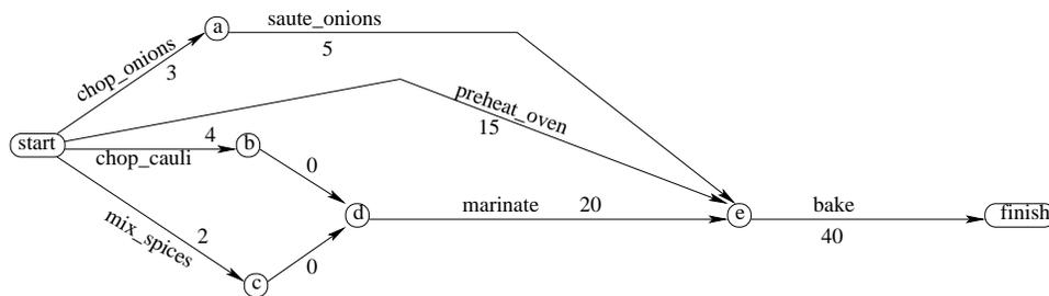
The longest tasks and the prerequisites relation are what determine the time it will take to complete the task. In this example, the dish will be prepared (at best) in 64 minutes. The path that determines this is “start” → “b” → “d” → “e” → “finish”. This is called the *critical path* and as you can see is the longest one from “start” to “finish”.
