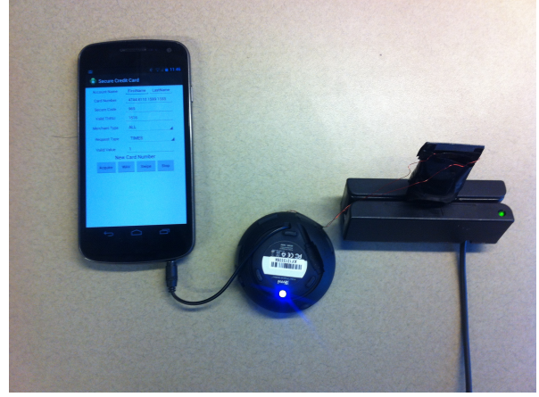
Fig. 5. A Picture of Our Prototype System (In real-world implementation, the amplifier and the solenoid can be combined together into one single chip, which can be directly plugged into the audio jack without a wire or connected with the phone through bluetooth).
