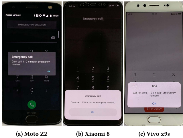
Figure 3: F-4: UEs which cannot identify emergency numbers of China (e.g., 110) when foreign SIMs are inserted.
