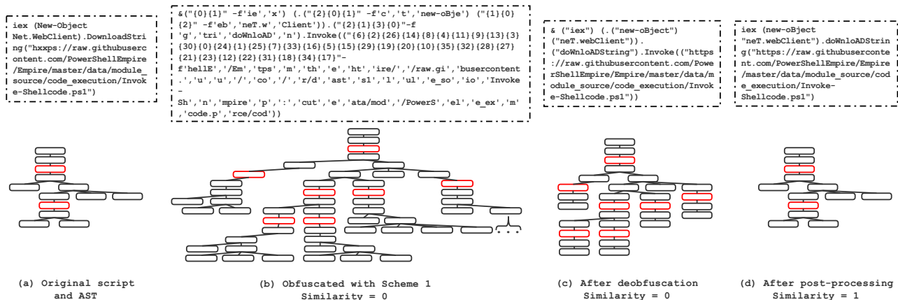
Figure 7: Effects of obfuscation and deobfuscation on the scripts and AST of an malware sample
