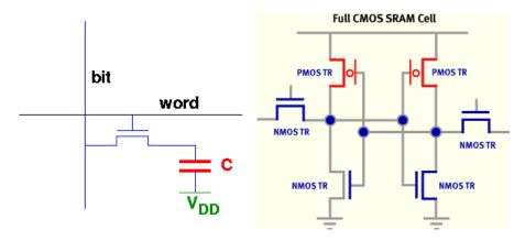
An important thing to notice is that an SRAM cell uses no capacitors but uses six transistors instead of just one. SRAM cells are much faster than DRAM cells, but also much more expensive. That's why they tend to be put in caches. An SRAM cell will also hold its bit as long as there is power. In a DRAM cell, because the bit is held in a capacitor and capacitors always leak charge, the bit must be frequently refreshed by external circuitry.
