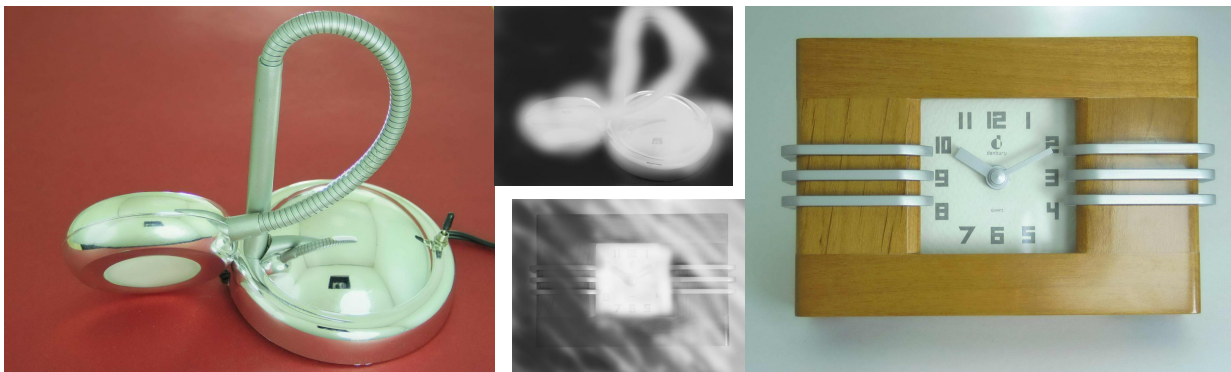
(d) Lighting a highly specular object by forcing the background to be dark.
