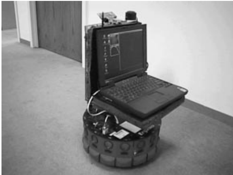
Figure 6: The hardware used by Cerebus. A commodity laptop with USB frame grabber, and NTSC board camera mounted on an RWI Magellan robot base.
