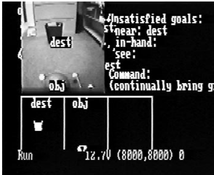
Figure 5: Kluge follows the command “continually bring green to blue.” The parser binds the object role to the color green and the destination role to blue, then asserts the goals in-hand(object) and near(destination). The robot grasps the green ball then drives toward the blue trashcan.
